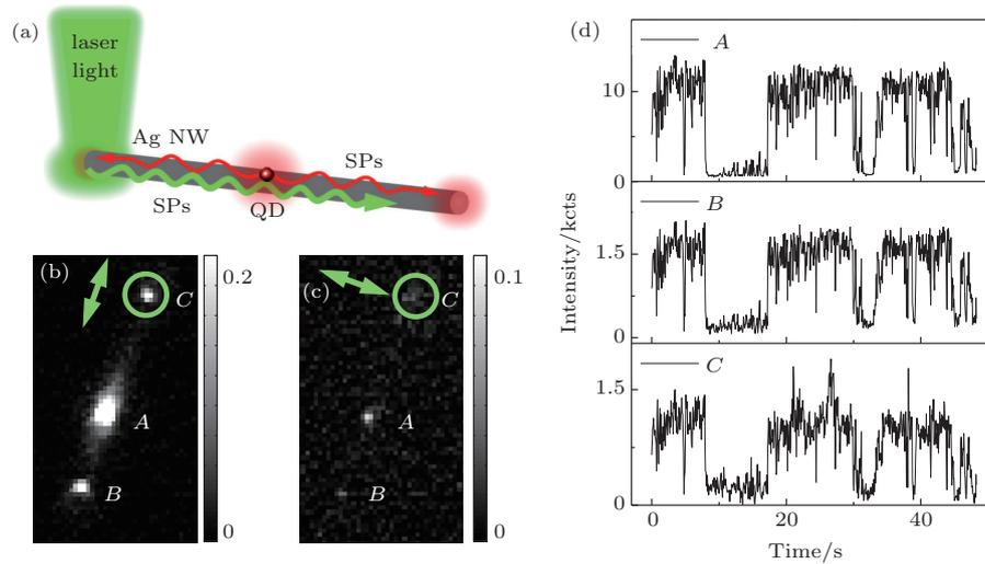
**Fig. 2.** (color online) (a) Sketch for remote excitation of a single QD using propagating SPs (denoted by the green wavy line) generated by focused laser light at the end of the NW. (b) and (c) Fluorescence images showing the remote excitation of QD A with laser polarization (b) parallel and (c) perpendicular to the NW. The green circles show the laser excitation positions. (d) Time traces of fluorescence counts of QD A and scattered light at B and C with the laser polarized along the NW.
