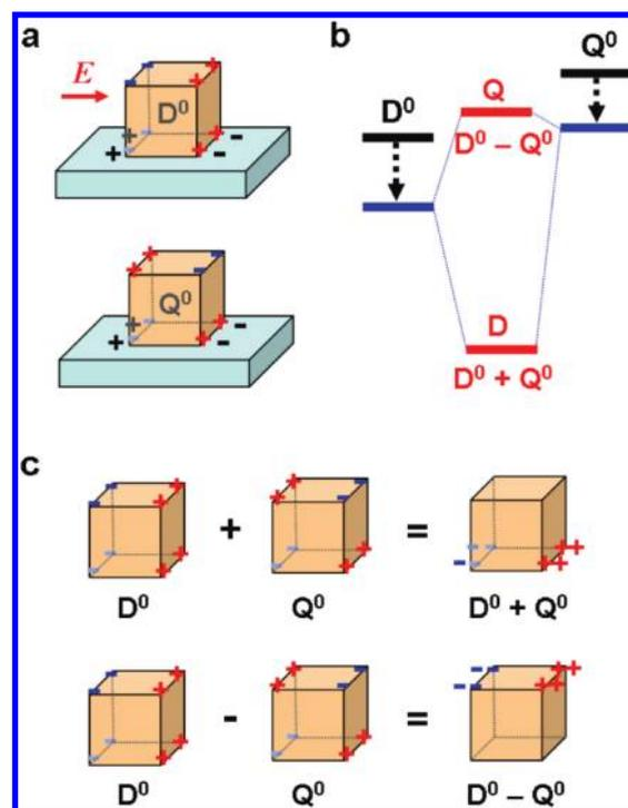
**Figure 4.** (a) Schematic illustrating the substrate-mediated  $D^0$  and  $Q^0$  interaction. (b) Energy diagram showing the substrate effect: pure dielectric screening effect (dashed black) which causes red shifts of both modes and the substrate-mediated interaction (thin blue line) resulting in hybridized bonding  $D$  and antibonding  $Q$  modes. (c) Schematic charge distributions of fully hybridized modes  $D = D^0 + Q^0$  and  $Q = D^0 - Q^0$ .
