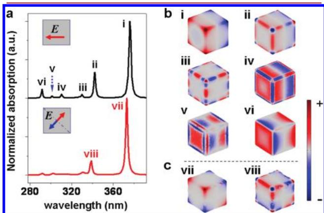
**Figure 2.** (a) Absorption spectra calculated using FEM and the DM for a 3 nm Ag cube in vacuum, excited by plane wave (black) and dark-mode excitation (red), as indicated in the inset. (b, c) Normalized surface charge distributions of the cube plasmon modes labeled in (a): (b) six bright primitive modes (i–vi); (c) two dark modes (vii, viii).
