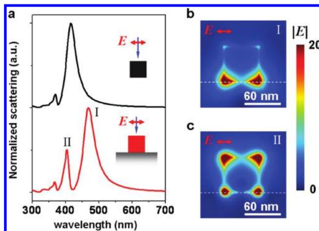
**Figure 1.** (a) Normalized scattering spectrum of a 60 nm Ag cube in vacuum (black) and on a glass substrate (red), under normal incidence plane wave excitation calculated using FEM and JC. (b, c) Electric field amplitude  $|E|$  at peak I (469 nm) and peak II (404 nm) in (a), at a plane 1 nm away from the side surface of the cube. The incident light is polarized parallel to the cube edge.
