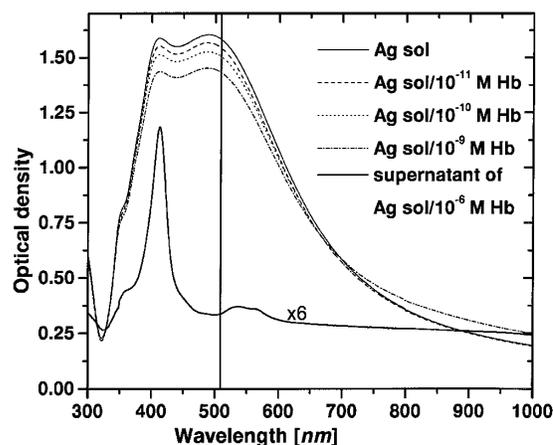
FIG. 1. Extinction spectra of Ag/Hb sols ( $[\text{Hb}] = (0-10^{-9})\text{M}$ ; 3 h incubation) together with supernatant Hb absorption after colloidal precipitation at  $[\text{Hb}] = 10^{-6}\text{M}$ . The vertical line marks the incident laser wavelength ( $\lambda_l = 514.5$  nm) used for Raman excitation.
