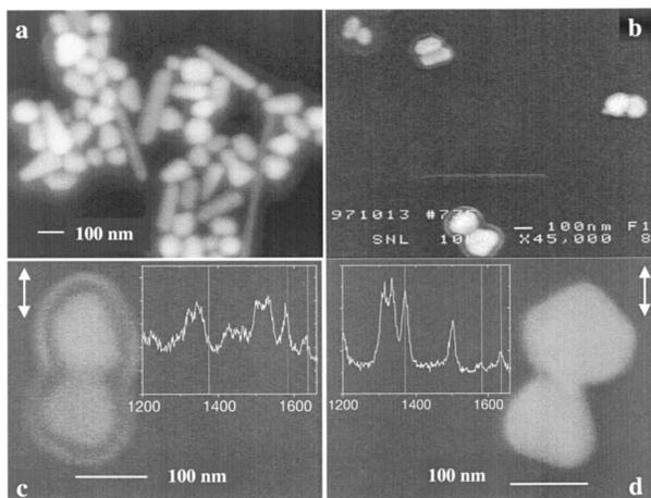
FIG. 3. SEM images of immobilized Ag particles. The pictures show (a) overview of Ag particle shapes and sizes, (b) Ag particle dimers observed after incubation with  $1 \times 10^{-11} M$  Hb for 3 h, and (c),(d) hot dimers and corresponding single Hb molecule spectra. The double arrows in (c) and (d) indicate the polarization of the incident laser field.
