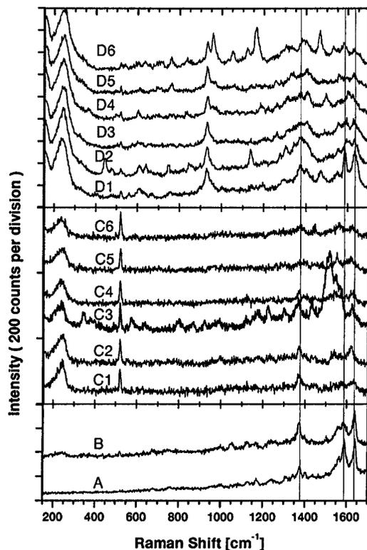
FIG. 2. Confocal Raman spectra of crystalline met-Hb (*A*), dense layer of Hb/Ag aggregates (*B*), and two time series (*C1*–*C6* and *D1*–*D6*) of “hot sites” obtained at the single molecule detection limit. The vertical lines indicate the Hb marker modes discussed in the text. All spectra were measured with the same collection time (30 s) and collection efficiency. The incident laser power was 1 mW in *A* and 1  $\mu\text{W}$  in *B*–*D*.
